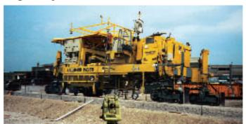
Guidance of shuttering machines, paver-spreaders, graders and milling machines. The advantage: The continuous on-line measurement with the total station eliminates the need for costly installation of cabling for controlling the machine.
